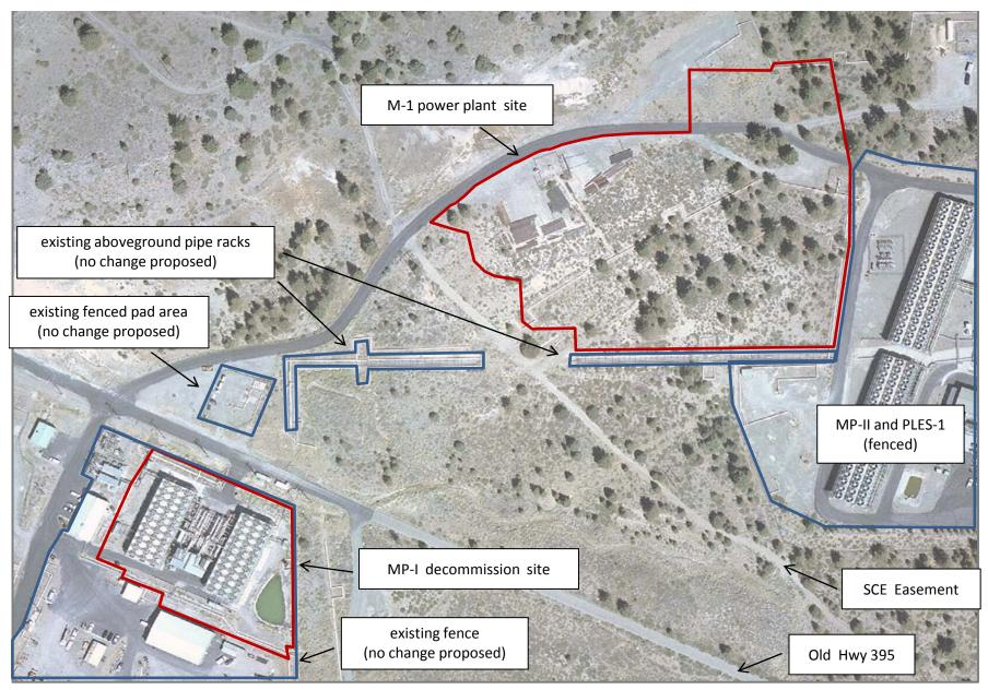
Figure 3. Position of the proposed M-1 Project elements (red outline) and adjacent geothermal energy production infrastructure (blue outline).
