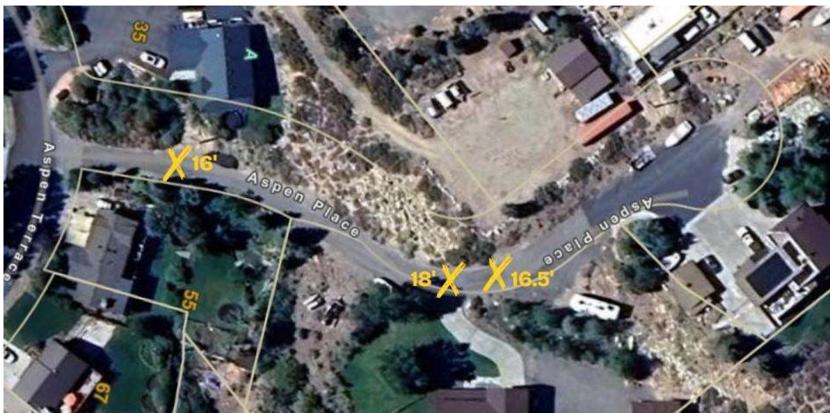
Figure 10: Road Width on Aspen Place
