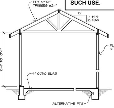
SNOW LOADING CRITERIA: 120 PSF SLOPED ROOF SNOW LOAD (C<sub>e</sub> = 1.0, C<sub>t</sub> = 1.2, I<sub>s</sub> = 1.0, C<sub>s</sub> = 1.0)
